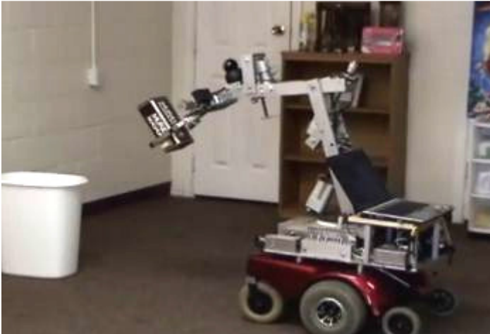
Figure 2 A Service/Research Robot Equipped with a Robotic Arm Manipulator
